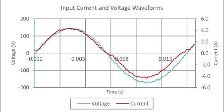
Note: All measurements were taken with input voltage at 115 V nominal at 60 Hz.
